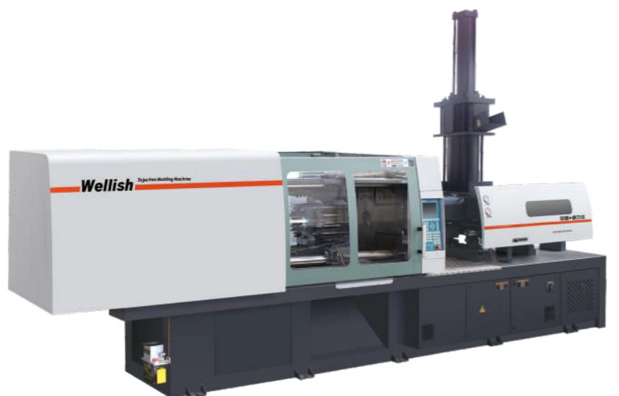
BMC injection molding machine is equipped with thermosetting physicochemical components which is specialized for BMC material. And it has system optimization module which is composed of specific charging automatic compressing device, specially high torque hydraulic motor for charging and special injection hydraulic cylinder etc.
